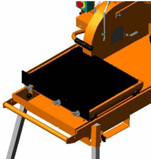
Figure 7: Conveyor Cart Installation
